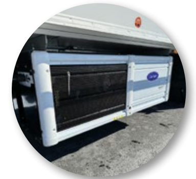
Chassis ramme montert kjøleaggregat
